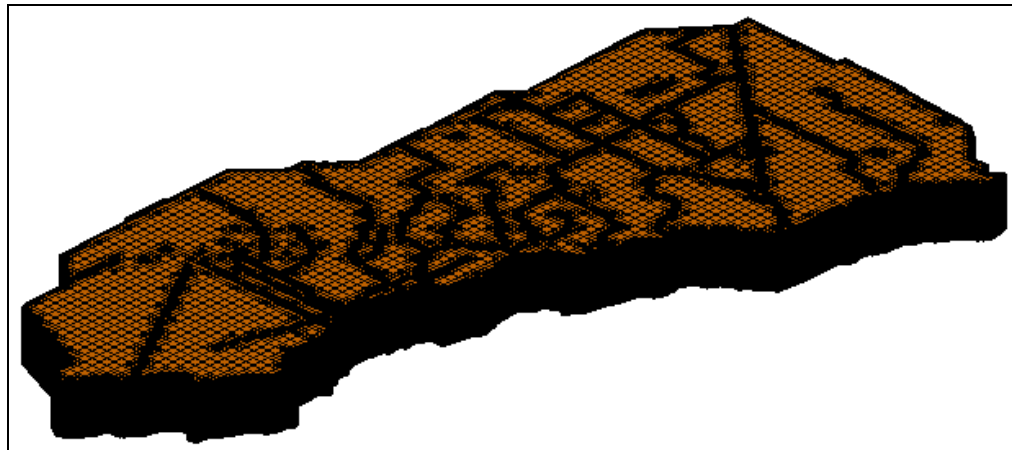
Figure 10 2D UGrid extruded to a 3D UGrid
