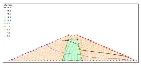
Figure 12 Contour lines after SEEP2D model run
