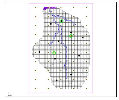
6. Using the **Create Scatter Points** •• tool, create a scatter point at each of the pumping wells as shown in Figure 6.
