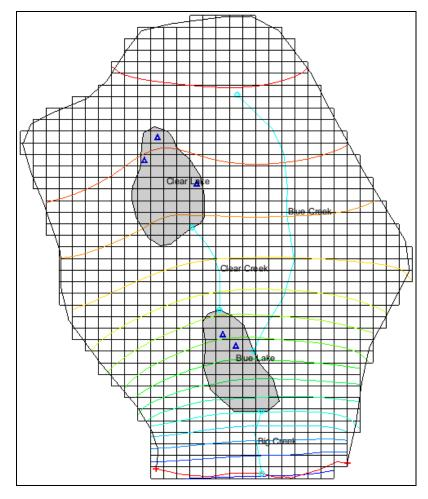
Figure 3 The computed solution after the MODFLOW run
